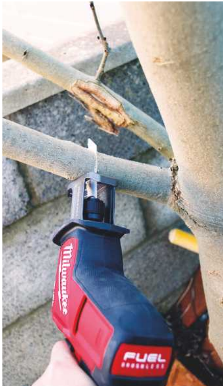
▲ The Quik-Lok collar makes blade swaps very, um, quick and easy
